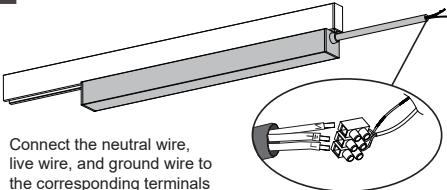
Connect the neutral wire, live wire, and ground wire to the corresponding terminals
