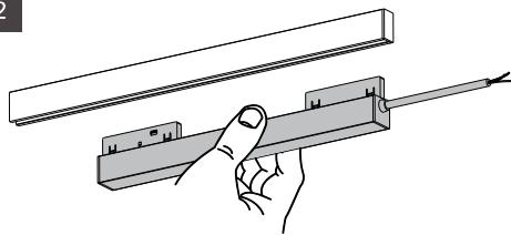
Align with the track and insert vertically
