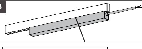
After installing the power supply, observe whether the power supply is firm and completely flat on the magnetic track with a "click" sound feedback
